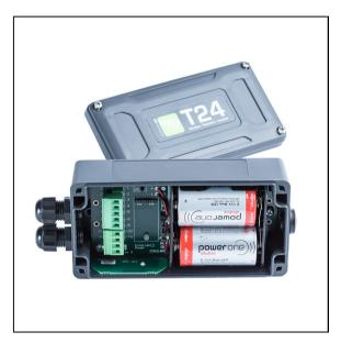
This remote loadcell data acquisition unit provides high performance wireless measurement of loadcell outputs. Providing direct mV/V input and 5V bridge excitation for up to 4 load cells. Low power modes allow the module to 'power down' between transmissions or to 'power off' completely and can be controlled by other T24 products such as the handheld displays or a base station.
